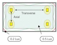
The diagram shows the area that needs to be covered for open area lighting. The main area is illuminated to a level of 0.5 lux. This excludes the area 0.5m away from the walls indicated by the dotted line.
