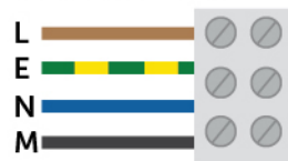
Maintained, 4 wires: Permanent live (L), Earth (E), Neutral (N), Switched live (M)
