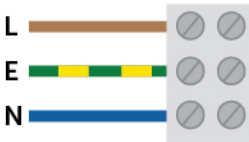
Non-maintained self-contained wiring
