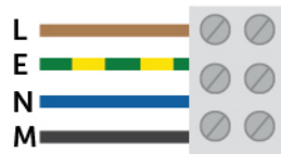
Maintained self-contained wiring
