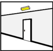
At every exit door planned to be used in an emergency.
