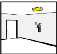
Near every fire safety device and call point.
